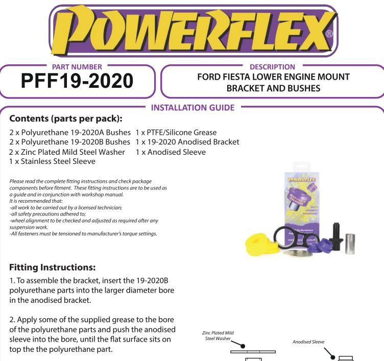
3. Insert the 19-2020A polyurethane parts into the other bore in the bracket.
