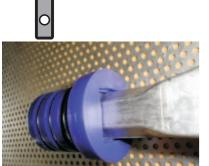
WITH CORRECT FITMENT METAL WASHER IN BUSH WILL SLIDE UP WISHBONE
