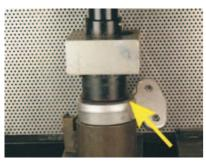
FIT OUTER PART INTO HOUSING SQUARE WITH PRESS, TAPER END FIRST **CHECK CORRECT WAY** ROUND
