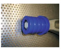
CORRECT FITMENT. SPIGOT FLUSH WITH END OF BUSH. **GREASE ALL AROUND OUTSIDE OF PURPLE** BUSH.
