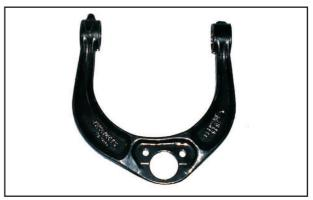
Photo 1. Cast arm with bushes removed.
