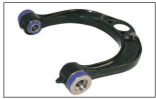
Photo 4. Cast arm showing complete bush assembly installed.
