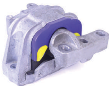
Figure 4 - showing all polyurethane inserts fitted inside the upper engine mount
