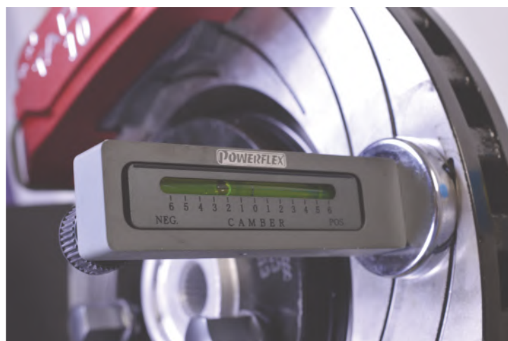
Figure 1 - magnetic camber gauge in use
