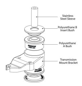
Figure 2: Exploded Assembly -Increased Rigidity
