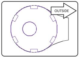
Fig 1. Maximum positive camber setting.
